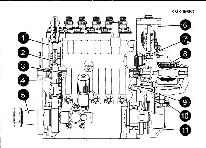
Further components in the RE positioner are an RPS (refer to system description for explanation of function), a contact connection plate with solder pins for the electrical connections of all components and (not always) an oil pump (viscous pump) for returning any oil which ingresses into the positioner to the camshaft chamber.
